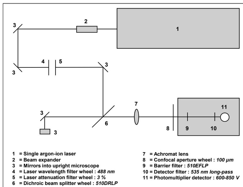
**Fig. 2** Schematic representation of the Sarastro-2000 confocal laser scanning system. See text for more details.
